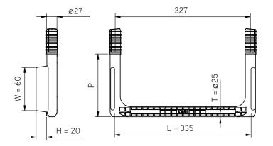
**Vertical load:** deformation  $\leq$  10 mm under a vertical load of 2 kN with permanent deformation  $\leq$  2 mm
