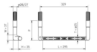
**Vertical load:** deformation ≤ 10 mm under a vertical load of 2 kN with permanent deformation  $\leq$  2 mm
